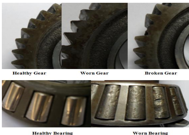
Figure 2. Different conditions of gear and bearing
